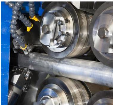
The new line is here part of a state-of-the-art plant producing semi-finished products, special bars for automotive forging and billets for extruding. The peeling machine operates in a diameter range of 50 – 203 mm with material lengths of 3 - 7 m and feed speeds up to 0,5 m/sec.
