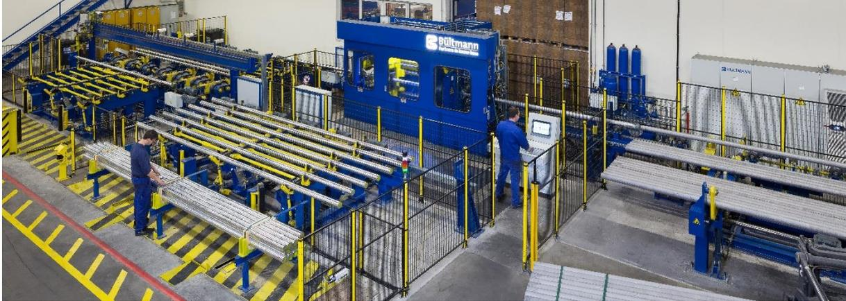
The recently newly developed BÜLTMANN high-performance peeling machines for aluminum bars, which successfully replace the extrusion of bars, are now well established with various customers, for example with one of the leading European suppliers of aluminum products and semi-finished products. With the help of the BÜLTMANN peeling machine, round billets are turned into homogeneous precision bars with high surface quality.
