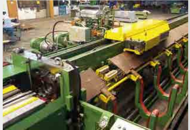
1-fach-Profil- und Stangenziehanlage für Messing- profile mit Push-Pointer Single profile and bar drawing equipment for brass material, equipped with push-pointer
