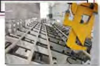
Beizhandlung zur Stangenziehanlage Handling system for bar pickling
