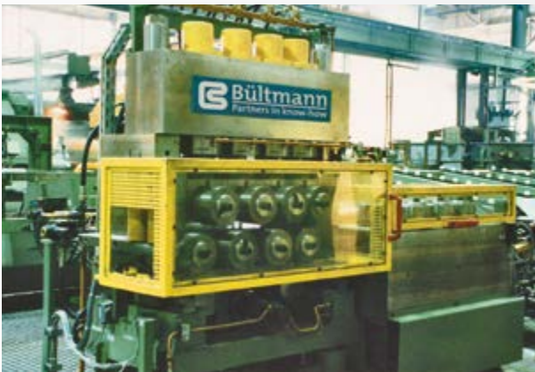
2 x 8-Rollen-Profilrichtmaschine für Messingstangen 2 x 8-roll profile straightening machine for brass bars
