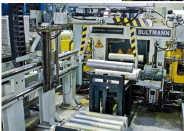
Bolzenbeladung zum MBH Billet charging system into the MBH
