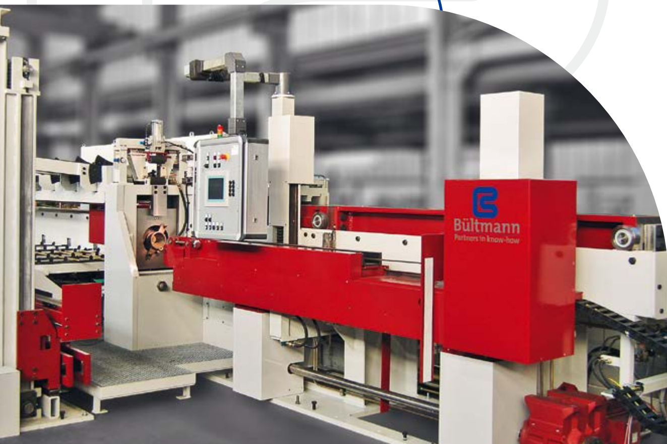
1-fach-Stangenziehanlage für Stangen aus Edelmetall Single drawing line for bars made of precious metal
