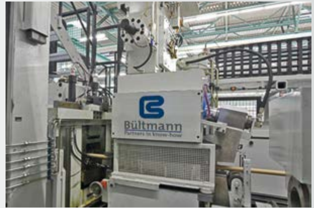
Push-Pull-Pointer in einer Ziehmaschine für Messing- stangen Push-pull-pointer on drawing machine for brass bars
