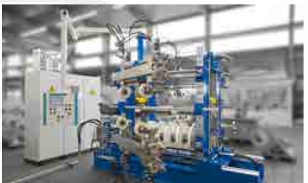
Mehrwalzen-Richtmaschine für Aluminiumprofile Multi-roller straightening machine for aluminium profiles
