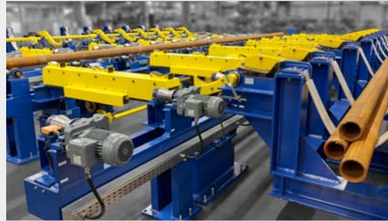
More than thousand driven V-shaped rolls ensure the longitudinal transportation of tubes.
