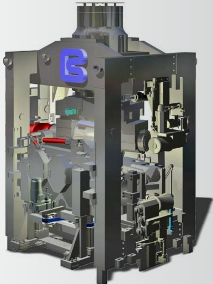
The centerpiece of the finishing line: 2-roll straightening machine with a weight of more than 400 tons.
