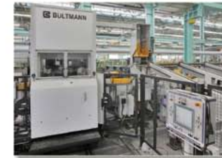
Rundstangenrichtlinie Straightening line for round bars
